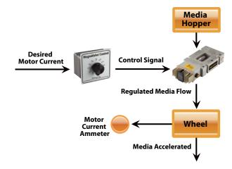
**Open Loop System** with Pot-24 Controller
