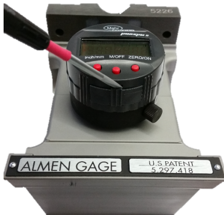
Figure 2. Open tray carefully with a flat blade screwdriver.
