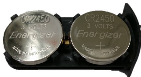
Figure 5. Batteries are placed with positive side up
