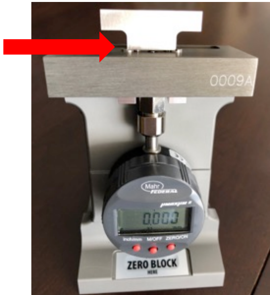
The small side of the Zero Block is placed on the gage. The reading is 0.000 mm.
