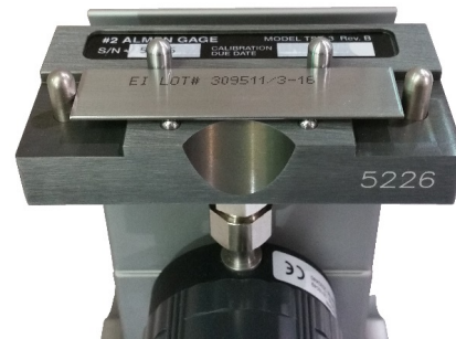
An unpeened Standard Almen strip placed on the #2 Almen gage.
