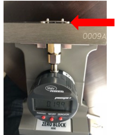
Peened mini-strip placed on the mini-strip gage. The reading is 0.199 mm.
