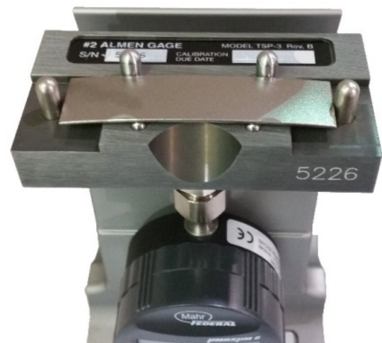
Peened standard Almen strip placed on the #2 Almen gage.
