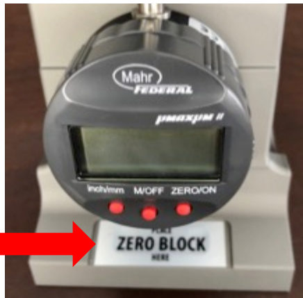
The magnetic base secures the Zero Block for easy access
