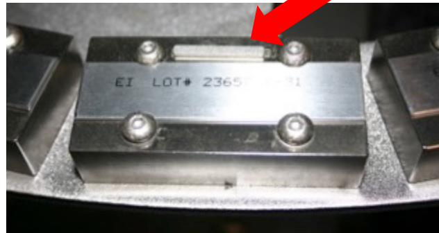
A mini-strip held in place with double-sided tape. This method should be used only when the mini-strip cannot be attached to the holder with screws.
