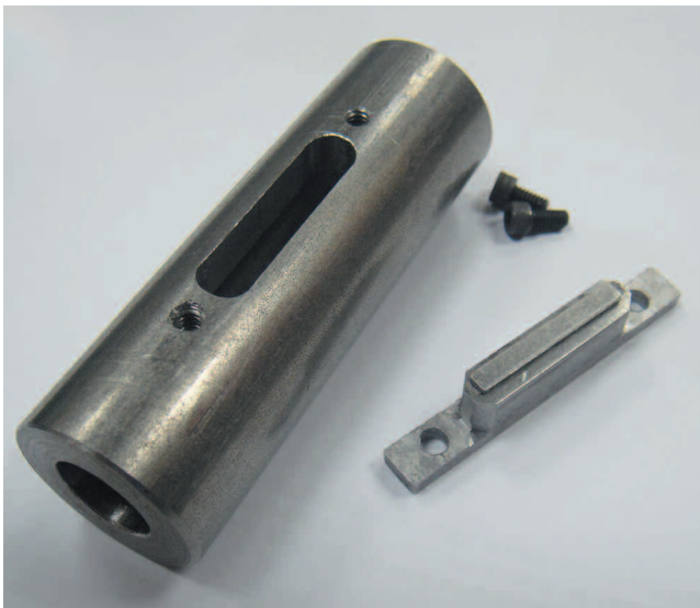
Shot peening technicians at Peening Technologies in Connecticut constructed this test fixture to simulate a component that requires lance-peening of a hole. To the left is an EI Almen mini-strip attached to a holder with double-sided tape. Above, the strip holder has been attached to the fixture with the mini-strip facing inside the pipe.
