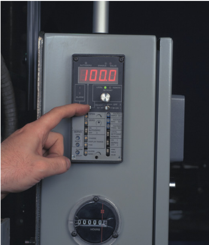
Figure 16. Original factory 100 amp setting
