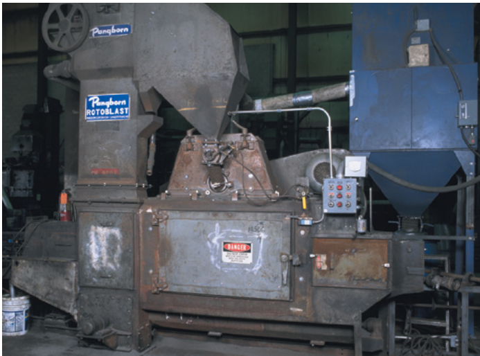
Figure 1. The Pangborn RotoPeen machine
