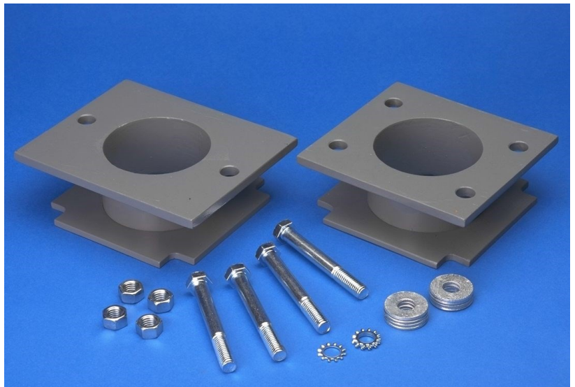
Fig. 9 Special adapter plates can be fabricated that will compensate for the bolt hole locations and vertical spacing needed by the MagnaValve.
