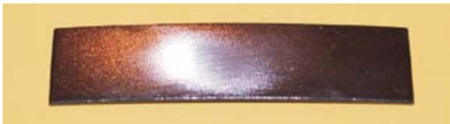
Fig.9. Hand-polished Almen 'A' strip showing area of complete indentation removal.
