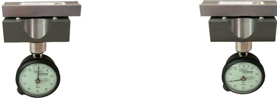
*Step Block Reading with the 0.015 inch step block.
