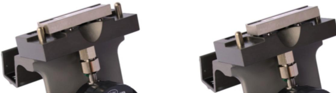
*Photograph on left: Place the step block to one side, allowing the indicator tip to touch the flat zero reference surface of the step block. Photograph on right: Slide the step block to the other side to allow the indicator tip to extend into the step.*
