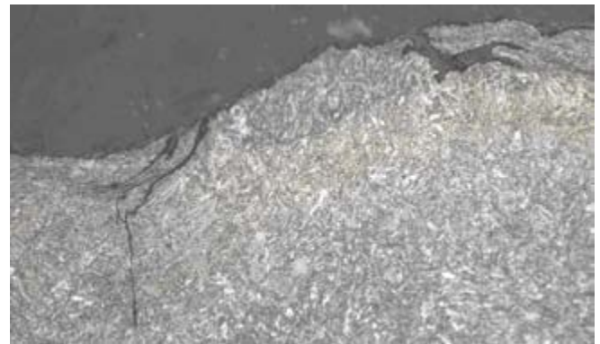
Figure 6. Fatigue Crack Emanating from Micro-Lap Surface Defect in AISI 5160 Spring Steel
