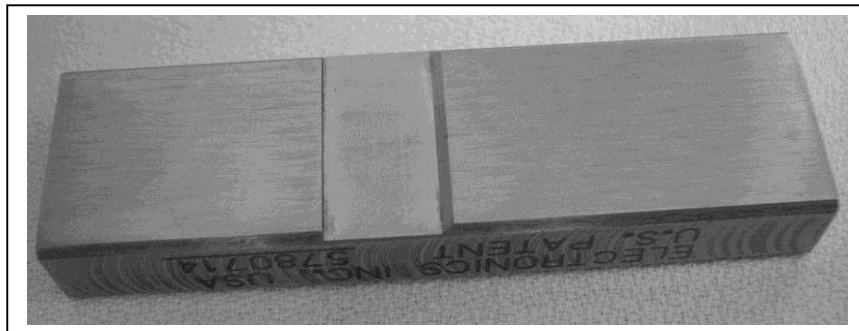
Figure 2a. Step block used to calibrate digital indicator
