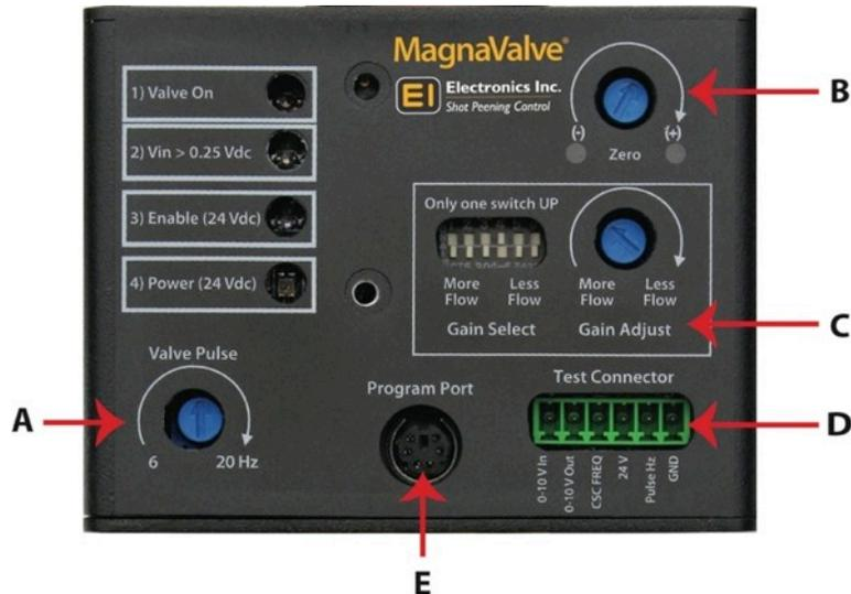
**A) Valve Pulse** – The rate at which the valve dispenses shot, similar to a heart beat rate. It is factory set to match the best flow characteristics of the media (cast steel, cut wire or micro-bead). Typical operation is set at 8 Hertz.
