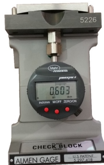
Figure 5. Place the curved side of the Curved Check Block on the gage
