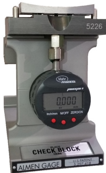
Figure 4. Place flat side of the Curved Check Block on the gage
