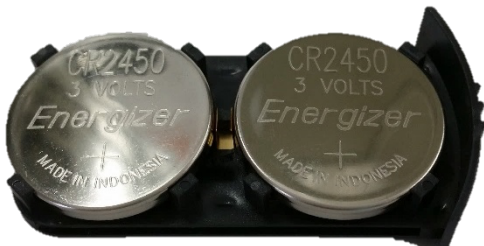
Figure 12. Batteries are placed with positive side up.
