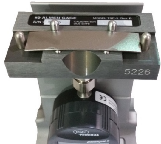
Figure 7. Place strip onto gage with indicator tip touching the non-peened side of strip
