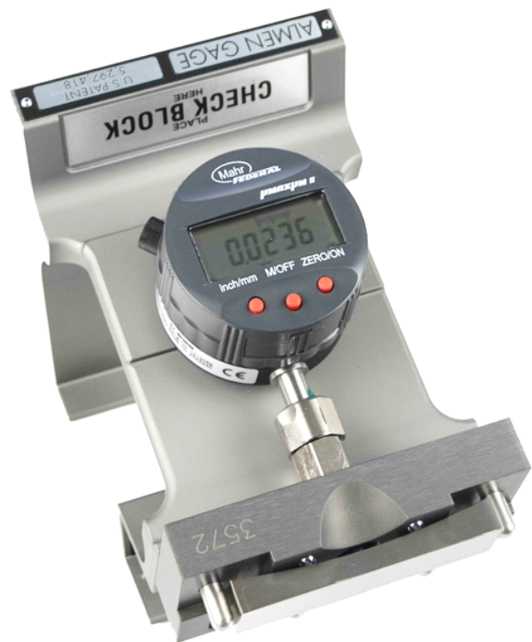
Figure 2. Gage shown when in standing position with Curved Check Block in measuring position (Display in inch mode).
