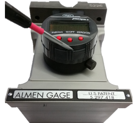
Figure 9. Open tray carefully with a flat blade screwdriver.
