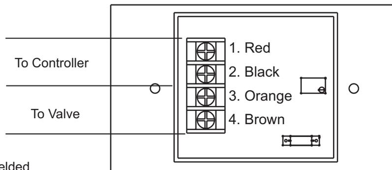
CABLE: 2 Conductor Shielded
