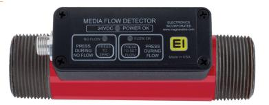
The MFD-P1 Sensor uses a charge-coupled amplifier that is connected to a sensing ring placed in the flow path of the abrasive blasting media. Each particle passing the ring shares a minute charge with the ring, converting it to a voltage used to activate the output relay contact.
