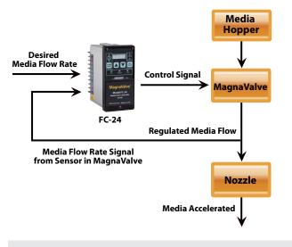
The FC-24 Controller is compatible with these MagnaValves:
