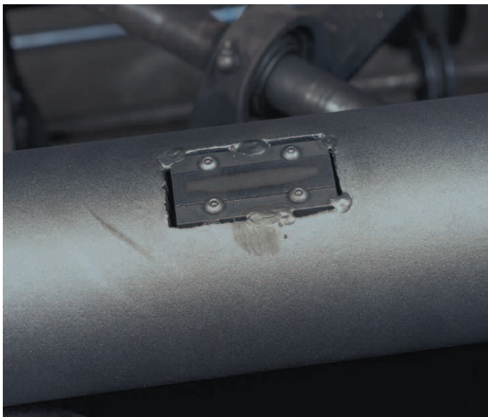
Figure 20. Almen strip attached to pipe
