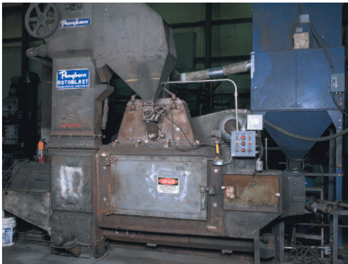
Figure 1. Pangborn RotoPeen machine ready for MagnaValve
